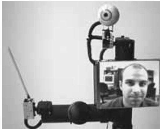
Figure 15.6. Closeup view of PRoP upper body with head and hand. Courtesy of the authors.
