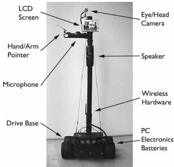
Figure 15.5. A PRoP with movable camera head, video, LCD screen, controllable “arm/hand” pointer, microphone, speakers, and a drivable base. Courtesy of the authors.
