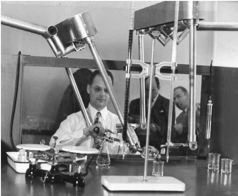
Figure 14.5. Photo of Ray Goertz and Telemip System. Ray Goertz, inventor of the first teleoperator. Source: Argonne National Laboratories public info office, Ms. Pat Canneday, 630-252-5562.
