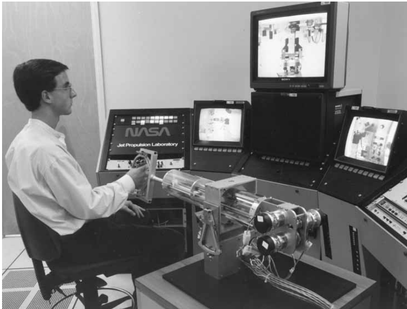
Figure 14.8. K. Salisbury 6 degree of freedom teleoperator. This device provided feedback forces and torques in all directions necessary for positioning and constraining an object in space. Source: JPL negative number 9647 Ac
