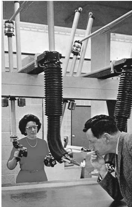
Figure 14.4. The original telemanipulators were mechanical devices engineered to handle toxic materials in the nuclear weapons complex. Source: Novelty postcard book published by Klutz press, 2170 Staunton Ct., Palo Alto, CA 94306 ( http://www.klutz.com ) — originally from Central Research Laboratories, Red Wing Minn. ( http://www.centres.com )
